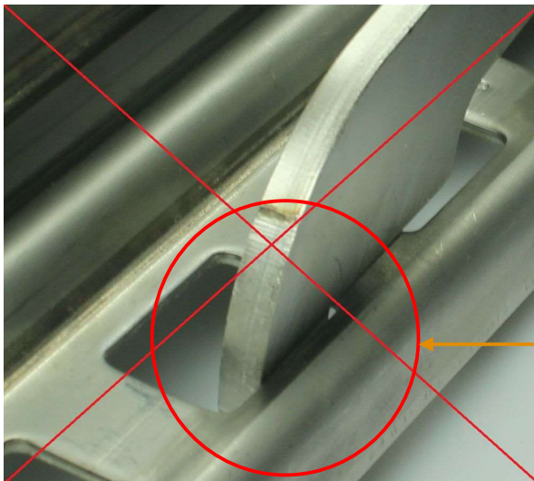
Incorrect position of the brake in the Frigowall track
